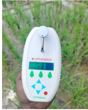
Fig.2 Opti-Sciences Chlorophyll meter (CCM 200 Plus)
