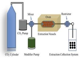
**Extraction:** The prepared material is placed in an extraction vessel, and the supercritical fluid, often CO<sub>2</sub>, is pumped into the vessel at high pressure. As the pressure and temperature are raised above the critical point of CO2 (31.1°C and 73.8 atm), it transitions into a supercritical state, where it exhibits properties of both a gas and a liquid. In this state, the supercritical fluid penetrates the material, dissolving the target compounds selectively.
