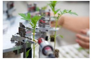
The first grafting robot, the "Cutting-off Cotyledon Grafting" (CCG) system, was developed in Japan by IAM BRAIN for cucurbits,
