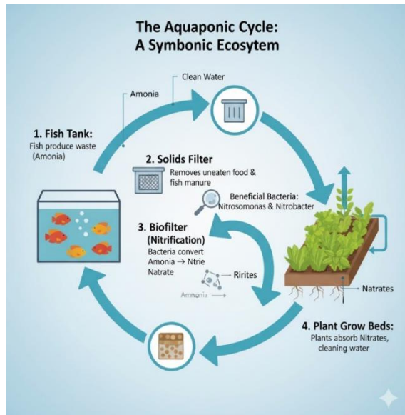
Fig: Aquaponic cycle: fish tank → solids filter → biofilter → plant grow beds → fish tank.
